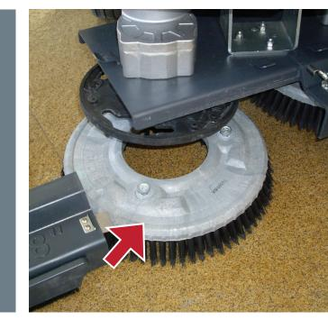
**1** Check if the brushes are correctly installed and not worn out.
