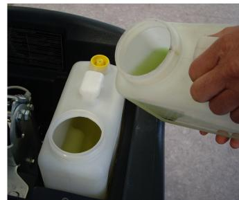
3. Fill the EcoFlex tank with a detergent suitable for the work to be performed (highly concentrated detergent).
