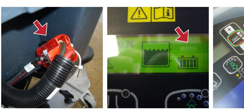
**1** Check if the power cable is correctly **2** Check if the battery is charged. connected.
