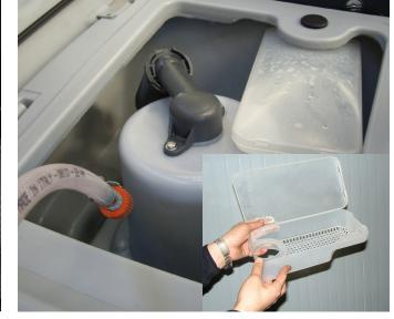
13. Wash with clean water the recovery tank and the vacuum grid. Remove and clean the debris tray.
