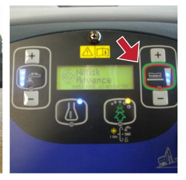
Check if there are external materials **4** Check if the Leds are on. Wait until the lights are steady.
