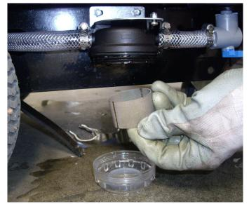
14. Clean the filter: 1) Close the solution tap under the machine. 2) Remove the transparent cover and the gasket, then remove the filter strainer.
